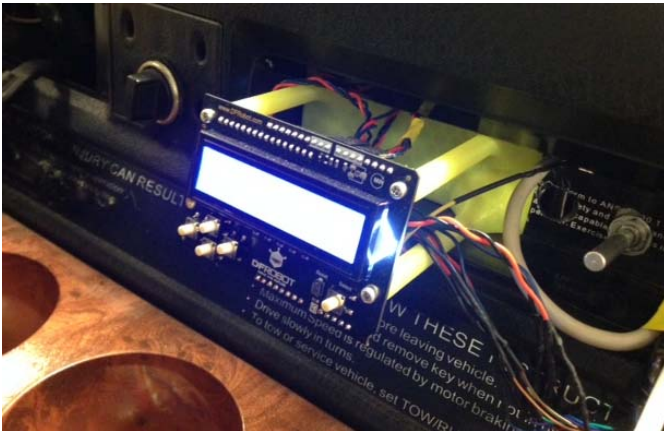
Figure 5. New LCD with 3D-printed mount
